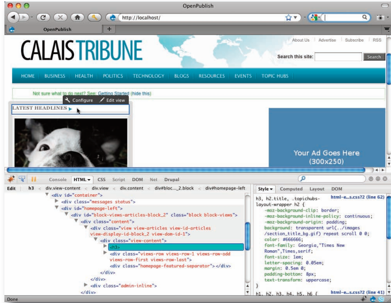
A Drupal page with the Firebug plugin showing CSS styles. The "Configure/Edit view" menu is a feature of OpenPublish, a version of Drupal optimized for publishers.
